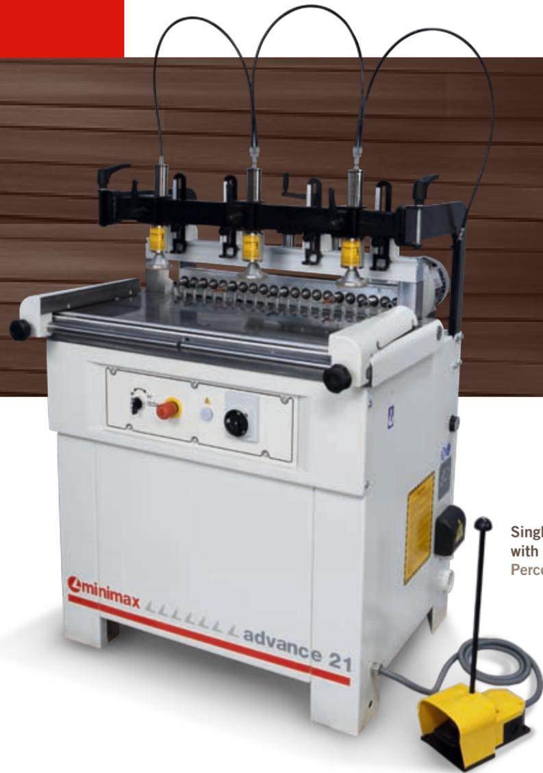
Single-head boring machine with 21 spindles
